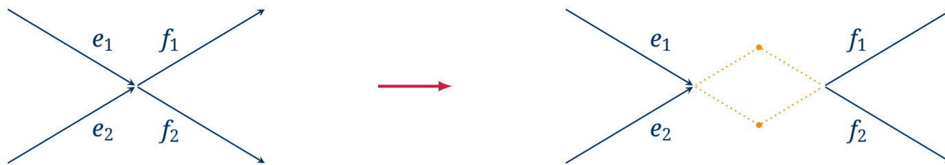
Figure 3. Given edge-disjoint paths P_1 = \langle e_1, f_1 \rangle and P_2 = \langle e_2, f_2 \rangle in G , the determinant of the matrix (I - X)^{-1}[\{e_1, e_2\}, \{f_1, f_2\}] enumerates this pair via the monomial \xi(P_1, P_2) = x_{e_1 f_1} \cdot x_{e_2 f_2} . The variables in this monomial provide enough information to uniquely recover P_1 and P_2 . In contrast, for k = 2 , the determinant of (I - YZ)^{-1}[\{e_1, e_2\}, \{f_1, f_2\}] assigns this pair weight
