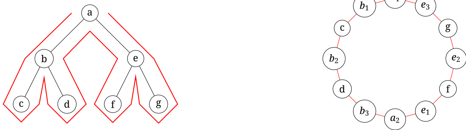
Figure 1. (Left) For the pictured \text{MST}(H) , the red line around the outside of the tree traces the tour T = (a, b, c, b, d, b, a, e, f, e, g, e, a) . (Right) We construct H' by mapping the tour T to a spanning cycle on 2n - 2 nodes, making copies of nodes from H as needed.
